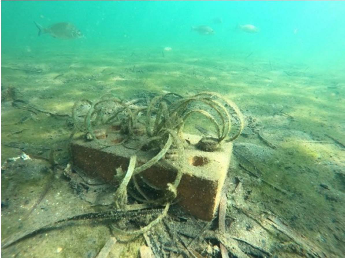
Figure 5 Pilot Seagrass ASU after four weeks immersion.
