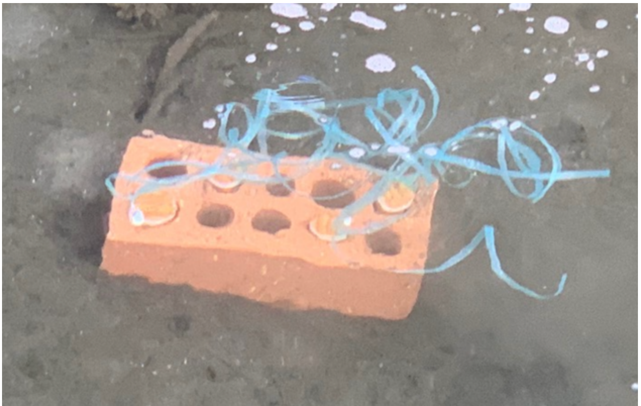
Figure 4 Pilot Seagrass ASU with four replicate Zostera ASUs at initial deployment.
