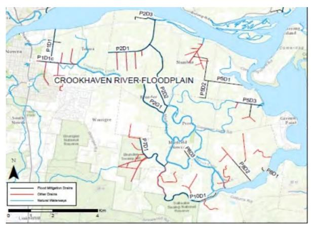
**Figure 6** Flood Mitigation Drains and Structures in Crookhaven River floodplains (from Glamore et al 2016).
